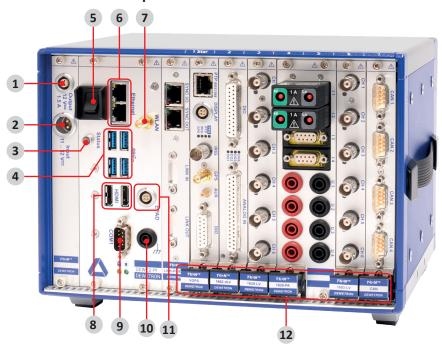
Fig. 4: Connections and ports DEWE2-M7s
