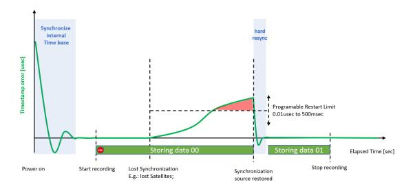
Fig. 15: Forced restart after restored synchronization
