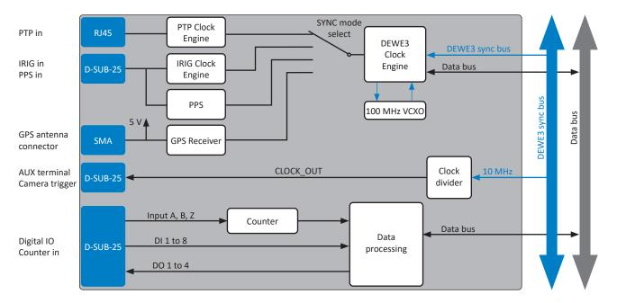
Fig. 13: Signal routing
