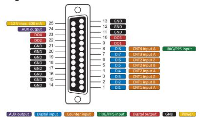
Fig. 7: Pin assignment D-SUB-25 connector
