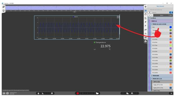
Fig. 24: Selecting instrument and signal
