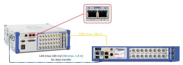
Fig. 28: Channel expansion with TRIONet
