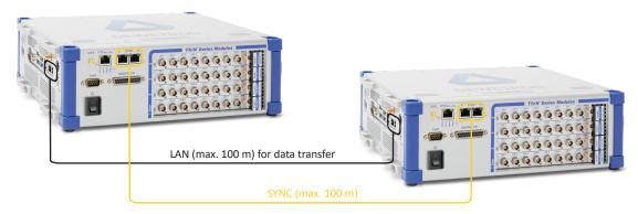
Fig. 29: Network with multiple systems
