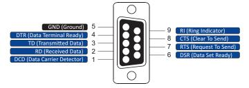
Fig. 11: Pin assignment RS-232 interface connector (COM1)
