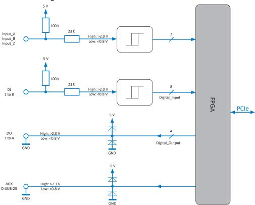
Fig. 9: Counter and digital I/O
