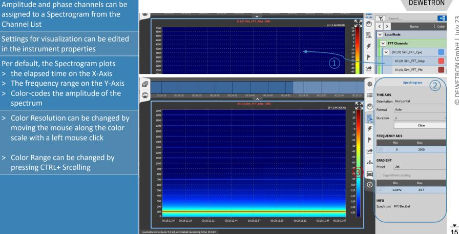
**Channel List** (2)Settings for visualization can be edited in the instrument properties Per default, the Spectrogram plots > the elapsed time on the X-Axis
