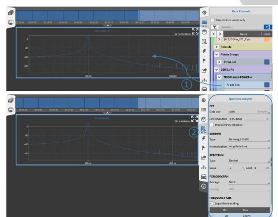
Possibility to directly assign time domain channels to a Spectrum Analyzer for FFT visualization
