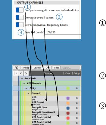
DEWETRON The actual CPB spectrum (changing in time) is calculated per default. The channel name is CPB
