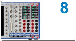
Pull up the injector/ejector handle to latch the module. Tighten the screws at the top and bottom of the TRION-1820-POWER-4 module front panel (4x) to secure the module.
