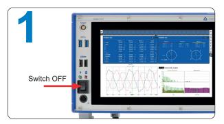
Switch off the instrument and unplug all connected cables including sensors from the TRION  $^{\text{TM}}$  series modules.
