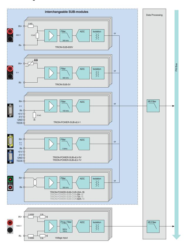
The TRION-1820-POWER-4 is an ultra-compact, 4-phase power data acquisition module with flexible current or voltage inputs for use in any DEWE2/3-chassis.
