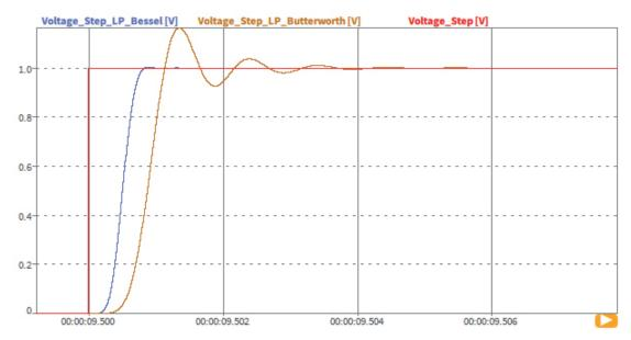
Figure 1: Step response of filter with 1000 Hz cutoff frequency and 8th order.
