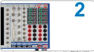
Loosen the screws at the top and bottom of the TRION-1820-POWER-4 module front panel (4x) and pull down the injector/ejector handle to release the module.
