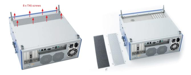
To clean the filter pad use a dry velocity stream of air. Afterwards, make sure to reinstall the louver and filter pad.
