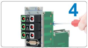
Loosen the torx screw (M2x4, TX6) which secures the sub-module of the channel you want to replace.
