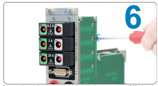
Secure the replaced sub-module with the torx screw (M2x4, TX6). Max. torque: 0.2 Nm  $\,$
