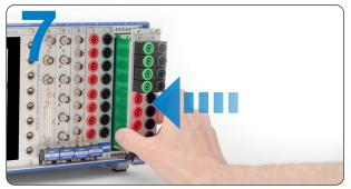
Insert the TRION-1820-POWER-4 module into the housing until a resistance appears.
