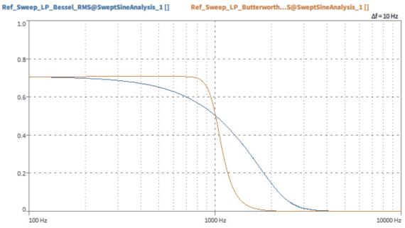
Figure 2: Frequency response of filter with 1000 Hz cutoff frequency and 8th order
