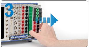
Remove the TRION-1820-POWER module from the housing.
