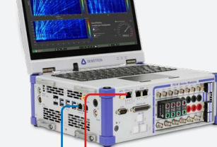
DEWE3-A4 with integrated PTP interface
