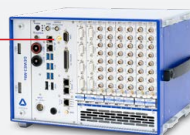
DEWE3-M8s with integrated GPS interface
